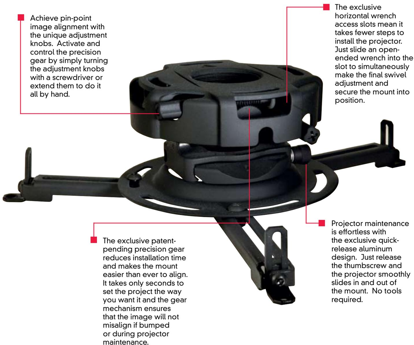
■ Achieve pin-point image alignment with the unique adjustment knobs. Activate and control the precision gear by simply turning the adjustment knobs with a screwdriver or extend them to do it all by hand.
