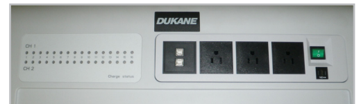
Led indicators and extra outlets on top
