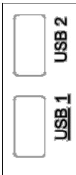
These 2 front bezel USB ports are routed to the 2 open USB cables on the rear of the panel. The cables have USB Type A connectors. They are used for connection to an optional computer if it is installed. They may be connected via a jumper USB extension cable to any of the USB panel ports or to an external computer.
