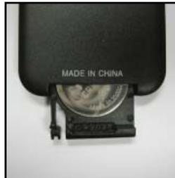
3. Place the clip back into the remote to complete the installation.
