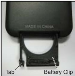
1. Push the tab, located on the left of the battery clip, to the right and pull out the clip.
