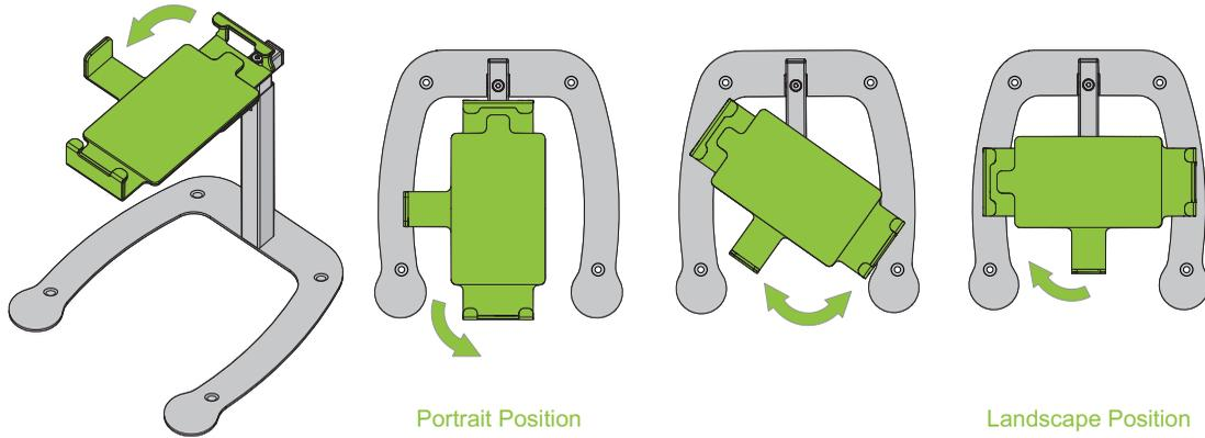
★ If swivel tension ever needs to be tighter, tighten this nut with 10mm wrench.
