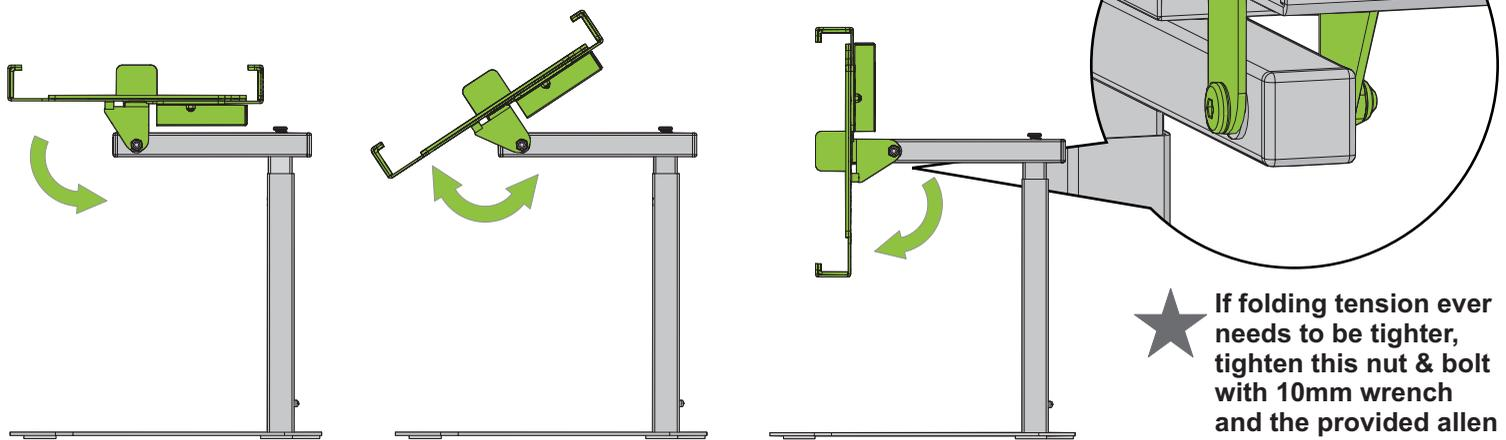
★ If folding tension ever needs to be tighter, tighten this nut & bolt with 10mm wrench and the provided allen
