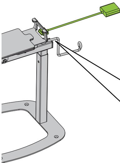
! To hold the VGA cable in place use provided VGA strap. Tie the strap around the adapter cable and then loop over the edge of the top mechanism.
