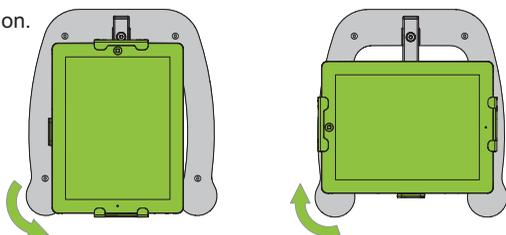
10. By tilting down the top mechanism, switch between document camera and stand position.
