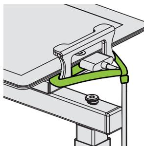
To hold the VGA cable in place use provided VGA Strap - Tie the strap around the VGA cable and then loop over the edge of the top mechanism.
