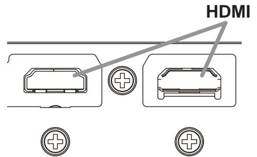
Remove the screw located on the lower side of **HDMI** connector and use it to attach the HDMI cable holder.
