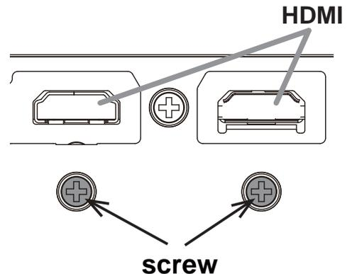
It is recommended to fasten the HDMI cables by using the HDMI cable holder and the Cable tie to prevent them from coming off. Use a Cable tie with the size of 2.0 x 4.0mm or smaller.
