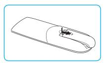
2. Install new batteries (AAA). Ensure that you have the batteries' polarity (+/-) aligned correctly.
