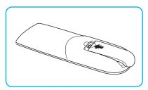
Note: Replace only with the same or equivalent type batteries.
